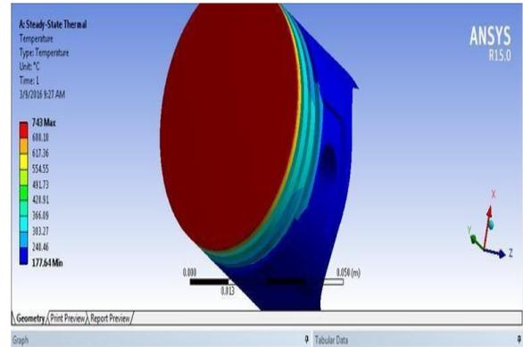
**Fig: 5.4 Temperature analysis on proposed Piston Face**
